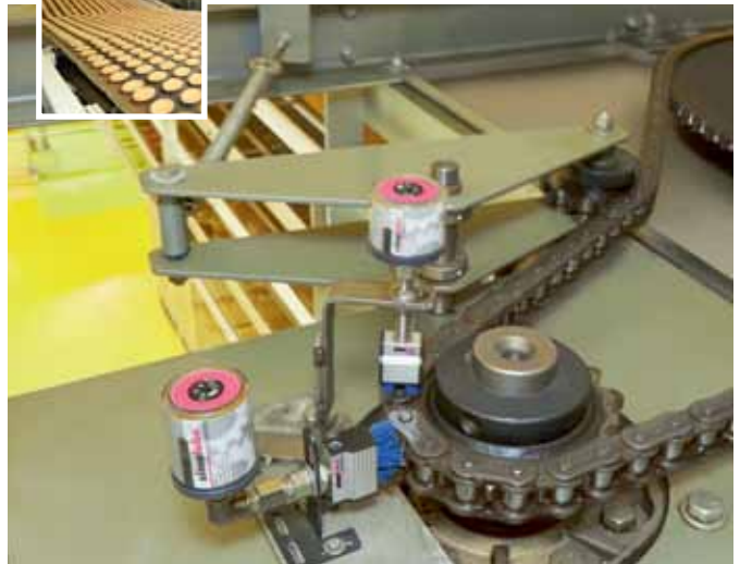
The drive chain of a transport belt, which allows rolls to cool, is cleaned with special blue brushes and lubricated with 2 simalube SL18 in 30 and 60 ml sizes.
